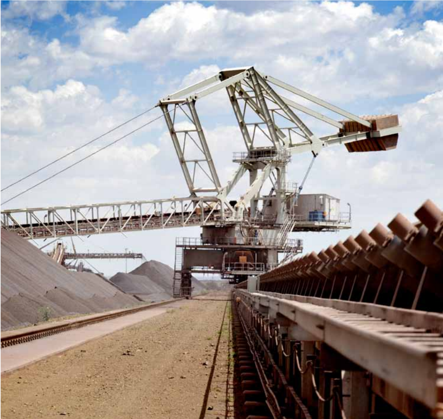
A stacker/reclaimer in operation in the final product yard of Khumani Iron Ore Mine.
