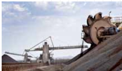
A stacker/reclaimer in operation in the final product yard of Khumani Iron Ore Mine.
