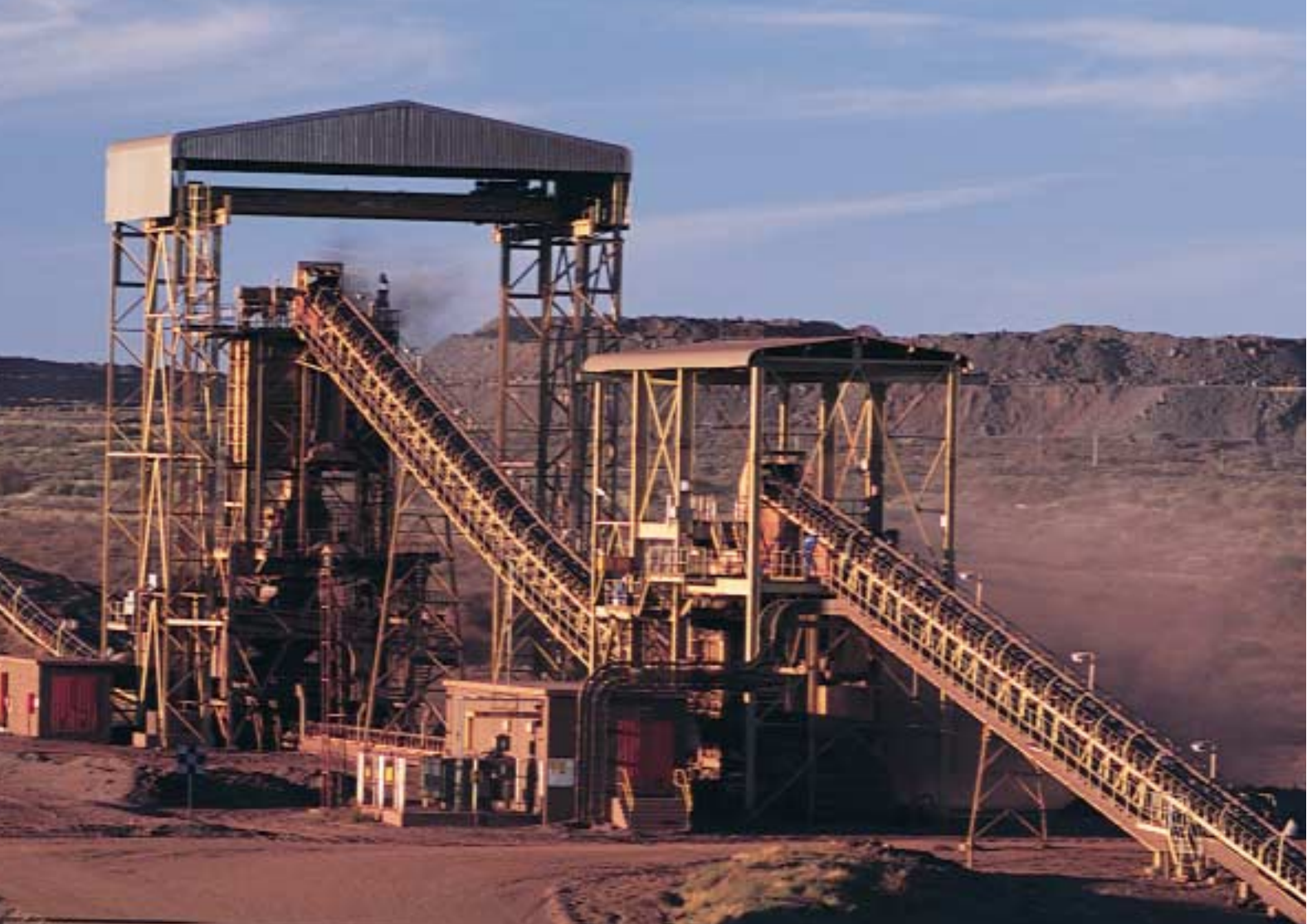
The primary and secondary crusher installation at the Beeshoek South iron ore mine from which the majority of the iron ore is produced
