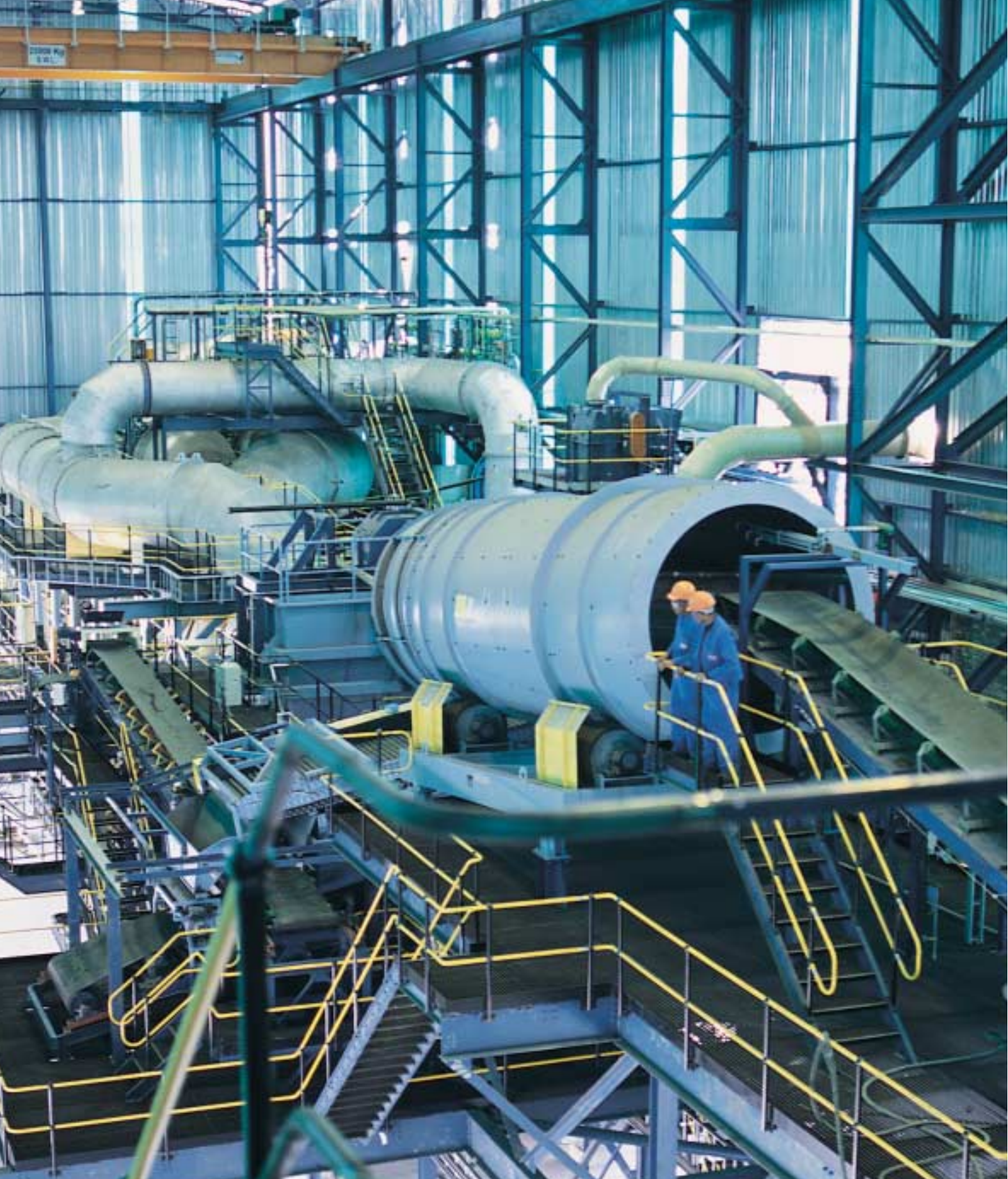
The pelletising drum section of the 350 000 ton per annum pelletising and sinter plant being installed as part of the chrome expansion project which will double chrome alloy capacity to 300 000 tons per annum
